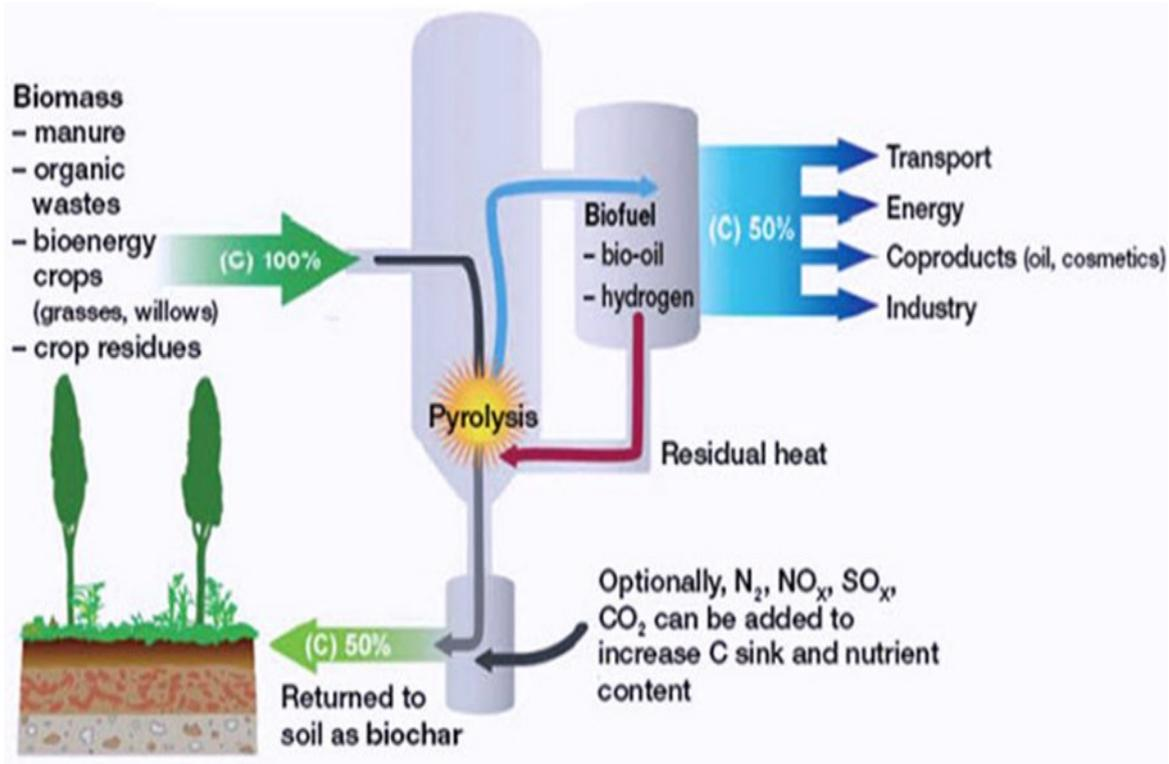
**Figure 1.** The diagram shows the pyrolysis process to produce biochar and syngas (Lehmann, 2007).
