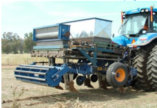
Figure 1 The 3-D Ripping Machine. The coulters in front of each ripping tyne and the back roller produce a flat seedbed.
